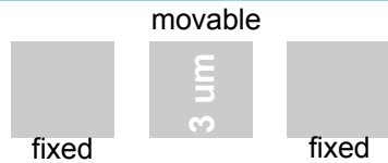
Today's finger cross section: no squeeze film damping
